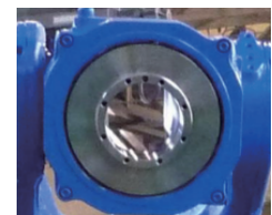
T-axis hollow arm: 50 mm dia.
