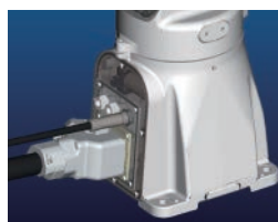
Power cable connection on the side and bottom (optional) of the manipulator
