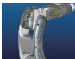
Built-in three-way solenoid valve (example of GP8)
