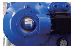
R-axis hollow arm: 50 mm dia.
