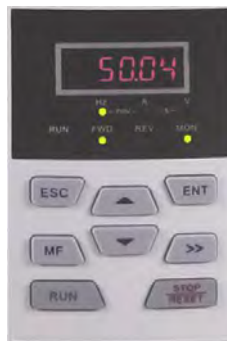
Fig. 4-7 Direct frequency modification status
