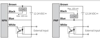
• The duration of a signal over 2 ms is necessary for the external input function. For using the external input, use a photocoupler or external controller, etc. Otherwise, it may result in product damage.
