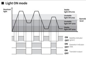
• In Dark ON mode, the waveforms are reversed
