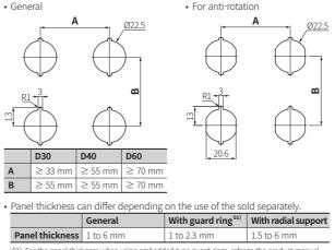
01) For the panel thickness when using embedded-type guard rings, refer to the product manual
