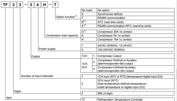
※1: Only for 1CH input, compressor output model (TF31-1□G).
