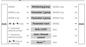
01) In the event of system anomalies and alarms, RESET input restarts the power controller. (parameters are not
